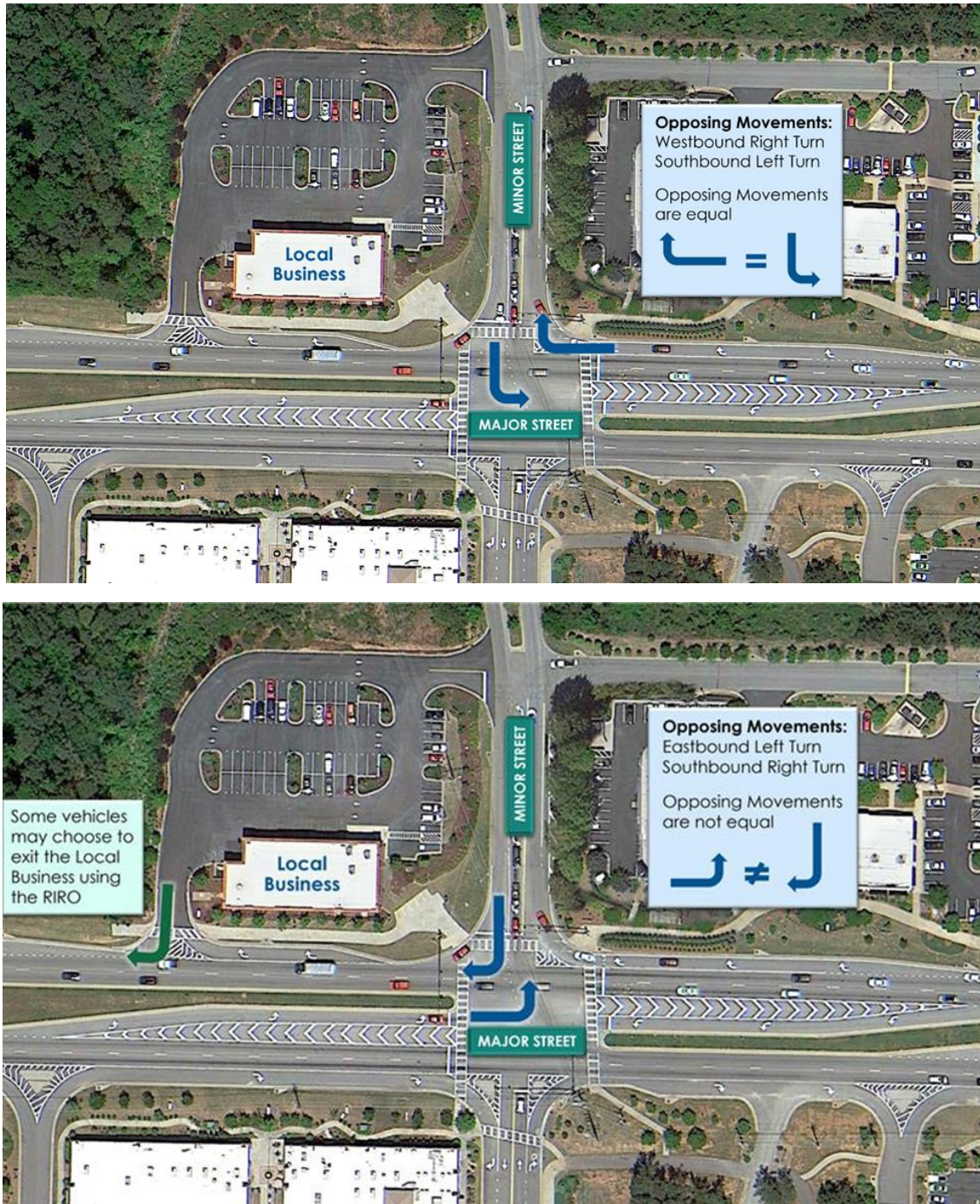
Figure 3.2. Example of AADT Balanced and Unbalanced Opposing Movements
